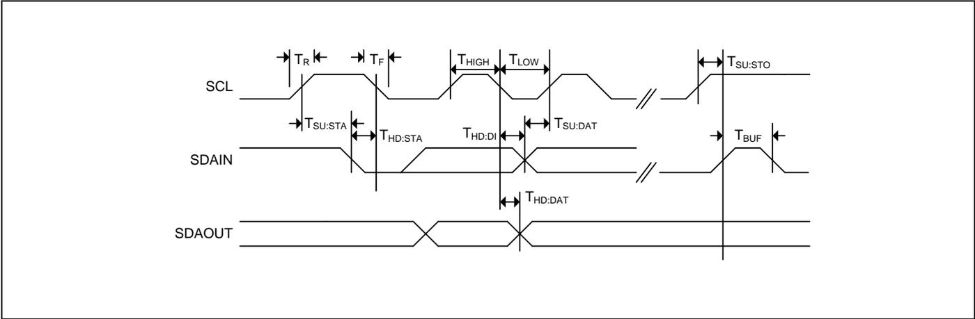
**Figure 5.7. Write Cycle Timing**
