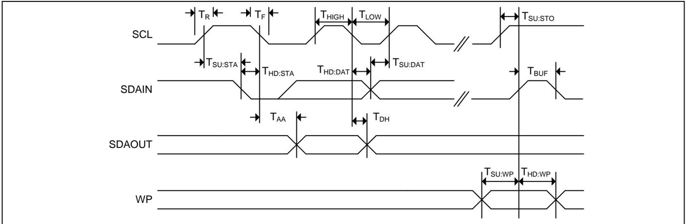
**Figure 5-7. Write Cycle Timing**
